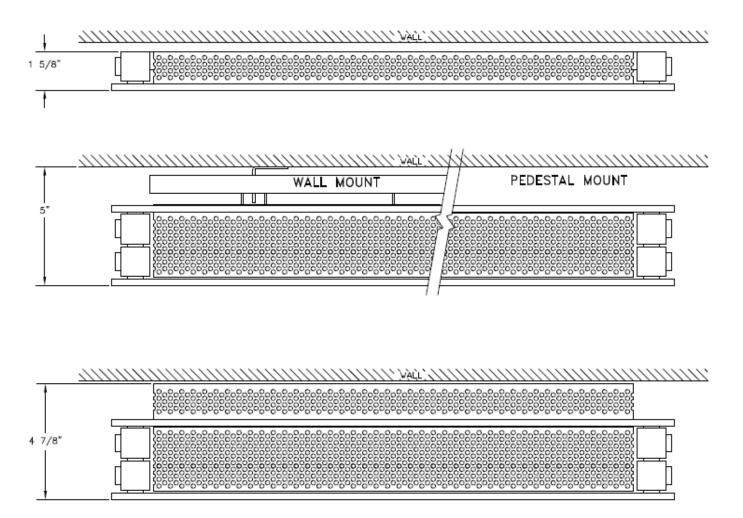
THE 16GA GRILLE WITH 3/16" DIAMETER HOLES ON 1/4" STAGGERED CENTERLINES PROVIDES A PENCIL PROOF FLAT TOP TO ANY STANDARD PANEL. THIS ALLOWS FOR A MORE CONTINUOUS LOOK AND PREVENTS UNWANTED BUILD UP BETWEEN THE FINS. THE GRILLE IS PAINTED AND FINISHED WITH POLYESTER EPOXY POWDER TO MATCH THE RADIATOR. ADDING THE PERFORATED GRILLE MAY REDUCE THE OUTPUT OF SOME MODELS.
