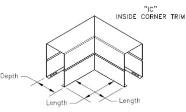
90° ANGLE STANDARD STANDARD LENGTHS 6" X 6" & 12" X 12" REQUIRED 2" MIN. OVERLAP 1 TUBE TO 4 TUBES HIGH
